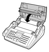
**10** If you replaced the film, initialize the new film by pressing the **FUNCTION** key, the "6" key, and the "#" key on the operation panel. Make sure that INITIAL-IZE FILM appears in the display, and then press the **START** key. (Do not perform this step if you installed the initial sample roll of film.)
